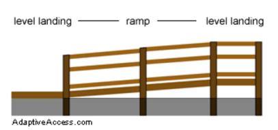
**R311.8.1 Maximum slope.** Ramps shall have a maximum slope of 1 unit vertical in 12 units horizontal (8.3 percent slope).
